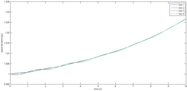
Fig -2: Change in generators speed without controls
