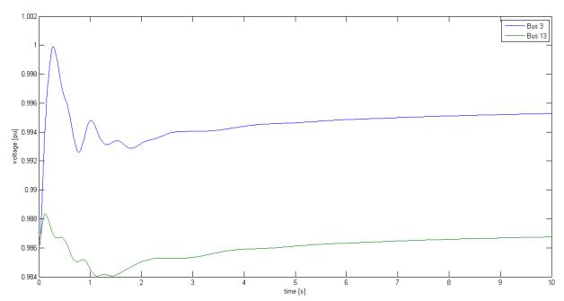
Fig -7: Change in Tie-Line Bus Voltage with PSS
