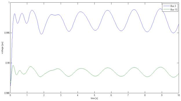
Fig -5: Change in tie-Line Bus Voltage with AVR & governor.
