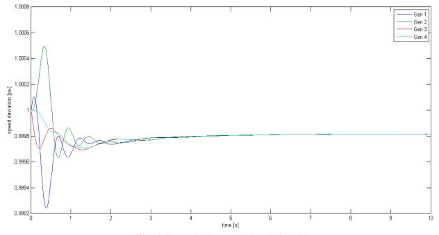
Fig -6: Change in Generators Speed with PSS
