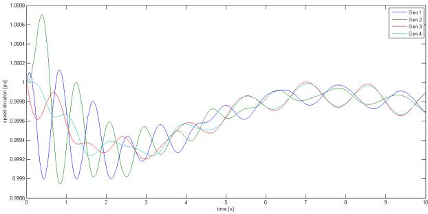
Fig -4: Change in generators speed with AVR & governor.
