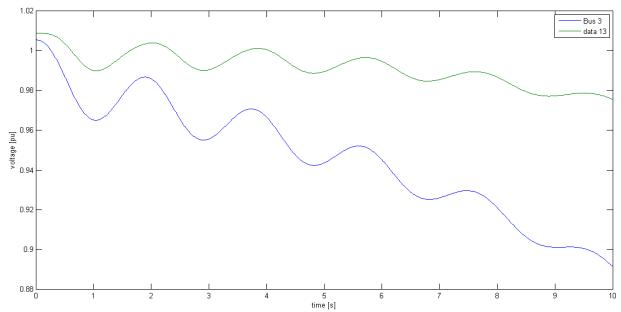
Fig -3: Change in tie-Line Bus Voltage without controls
